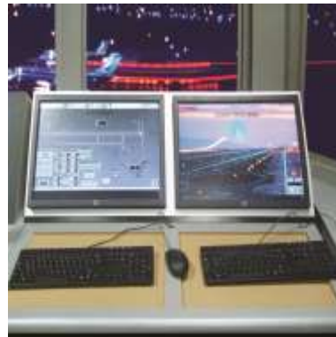
ALCMS Airport Lighting Control and Monitoring System
